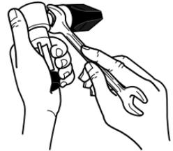
Tighten the transmitter by means of a size 19 wrench.
